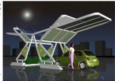
Each charging station is made of separated parts that can be assembled and erected on site. In that way the station can be shipped and assembled on site anywhere, on a low budget.
